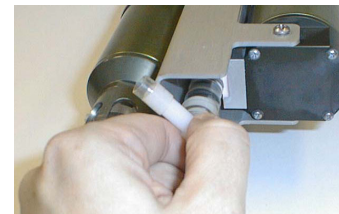
Temperature sensor guard rotated 90° counterclockwise while C Duct rotated clockwise slightly
