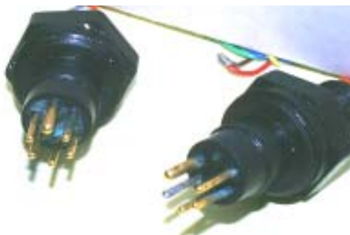
Corroded pins on bulkhead connectors - Connector on right has a missing pin
