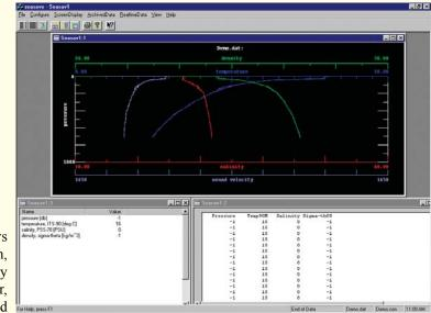
transmissometer). What if you are using an auxiliary sensor that is not directly supported by our software? Auxiliary sensor selection includes a user polynomial, allowing you to define an equation to relate your sensor output voltage to calculated engineering units.
