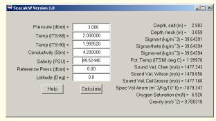
SEASOFT for Waves<sup>©</sup>-Win32 is a powerful modular program for use with the SBE 26plus (or older SBE 26) SEAGAUGE Wave and Tide Recorder or SBE 53 BPR Bottom Pressure Recorder. It includes:
