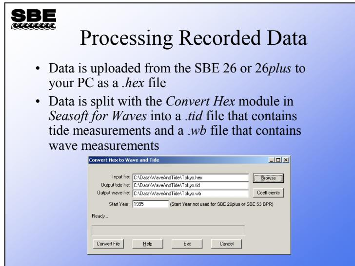
Data that comes from the SBE 26 or *26plus* has wave burst data embedded in the tide data. The first step is to split this data (*.hex*) into 2 files (*.tid* and *.wb*).
