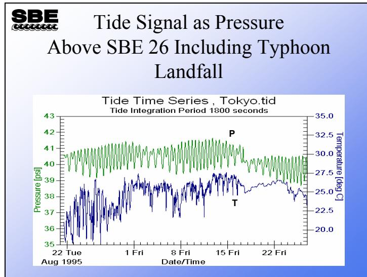
Our example data comes from Tokyo harbor. During this deployment a typhoon made landfall. In this deployment the SBE 26 was fixed in 18 meters of water and was 1 meter off the bottom. Wave bursts were 600 samples long (Why would this be a silly thing to do?).
