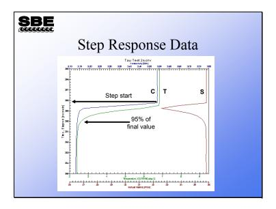
The above plot shows the results of the experiment. The Y axis is time in seconds; this corresponds to decibars at a lowering rate of 1 meter per second. Note that the temperature trace lags the conductivity trace, because the SBE 19*plus* temperature sensor time constant is approximately 0.5 seconds while the conductivity cell has a time constant of about 0.030 seconds.
