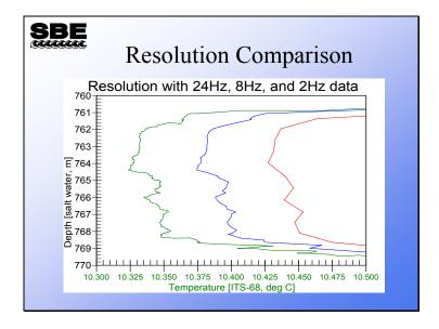
The left-most plot is data collected at 24 Hz with a nominal 1 meter/second lowering speed. The middle plot is the same data set decimated to 8 Hz to represent the resolution of the SBE 25. The right-most plot is the 24 Hz data set decimated to 2 Hz, which is representative of the resolution that would be seen with an SBE 19. The obvious conclusion is that a faster sampling rate yields higher resolution of temperature structure in the ocean temperature profile.
