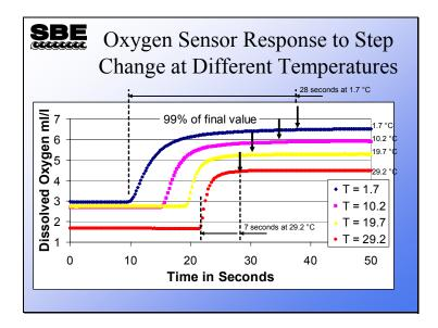
The plot above illustrates the effect that temperature has on a dissolved oxygen sensor. The colder the water that the sensor is working in, the longer it requires to come to a final value. This phenomenon is observable as upcast and downcast hysteresis. We will consider how to lessen this effect with the data processing *Align CTD* module in Module 9.
