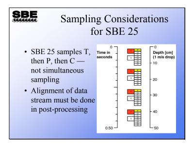
The SBE 25 has a different sampling order. The alignment of T and C must be done in post-processing, regardless of whether the SBE 25 is used for internally recording data or as a real-time instrument with a deck unit. As an internally recording instrument, the SBE 25 has the capability of averaging samples to increase the memory endurance. Averaging degrades the resolution of the instrument and makes the alignment of T and C less effective.
