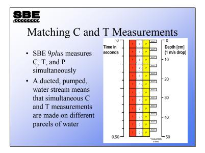
The SBE *9plus* acquisition architecture measures temperature, conductivity, and pressure simultaneously. Careful examination of the plumbing of the TC duct shows that a water parcel first encounters the SBE 3 thermistor and then transits into the conductivity cell.
