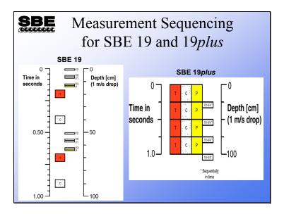
As was mentioned on the previous page, the SBE 19 samples P, then T, and finally C, at a sampling rate of 2 Hz. Because T and C use the same oscillator, there is separation in the measurements to allow time for the oscillator to settle into the new frequency after it has been switched. Alignment of T and C is done in post-processing and, as mentioned earlier, averaging of scans to improve memory endurance tends to degrade the instrument's resolution and make alignment less effective.
