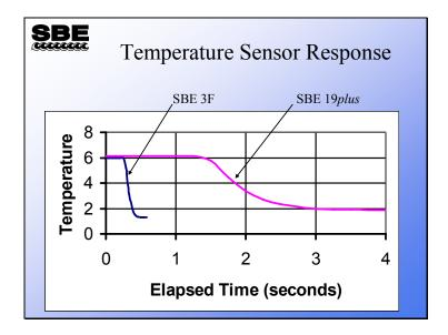
This plot compares the time response of the SBE 3F with the SBE 19*plus*. The SBE 3F has a smaller thermistor and a smaller needle, giving it a faster response time.
