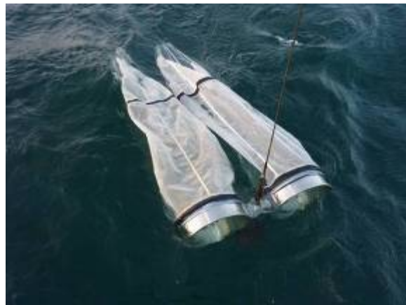
Horizontally towed Bongo 505 \mu\text{m} nets
