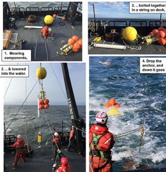
Steps for deploying a mooring - harder than it looks.
