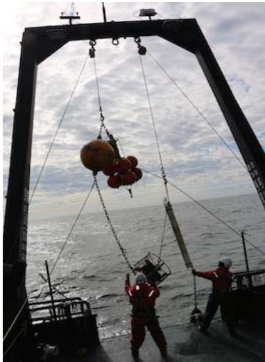
Using the winch, the mooring is lifted from the water onto the deck
