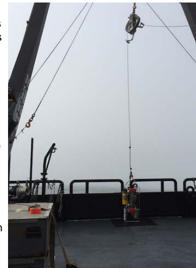
A lonely CTD sits on the aft deck of the ship in fog
