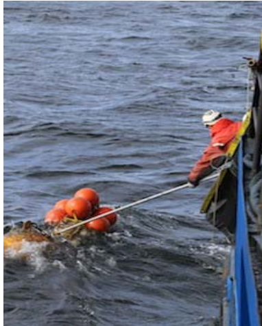
The crew hooks the mooring out of the sea
