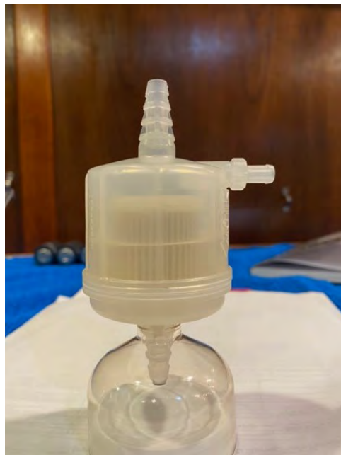
Clogged/used Acropak 200 (0.2um) filter. Top is the barbed connection that would be attached to the white C-flex tubing. To the right is the air valve that was opened during flushing to prevent bubbles from clogging the filter. Note that the folded Supor filter inside the capsule is dark green/brown after sampling.
