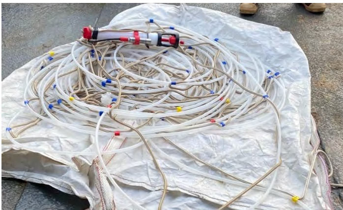
View of coiled rope and tubing with tape markings (left) and mini RBR CTD (red, white, black). Bucket used to collect unfiltered flow during flushing with shackle attached to restrict the “bouncing” of the white C-flex tubing that occurs due to the pump pressure.
