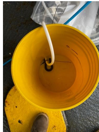
View of coiled rope and tubing with tape markings (left) and mini RBR CTD (red, white, black). Bucket used to collect waste flow during flushing with shackle attached to restrict the “bouncing” of the white C-flex tubing that occurs due to the pump pressure.
