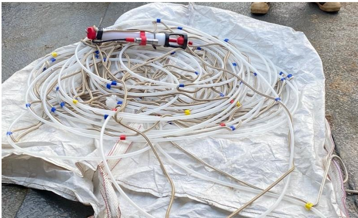
View of coiled rope and tubing with tape markings (left) and mini RBR CTD (red, white, black). Bucket used to collect waste flow during flushing with shackle attached to restrict the “bouncing” of the white C-flex tubing that occurs due to the pump pressure.
