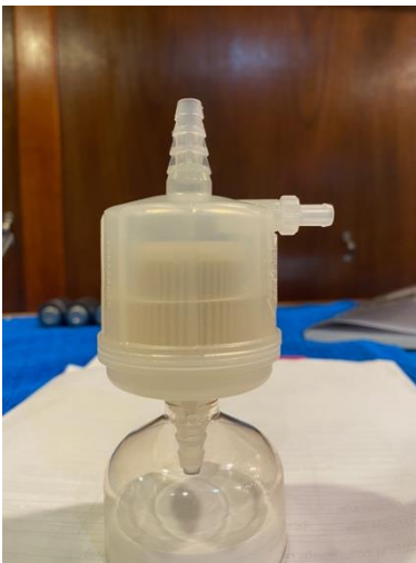
Clogged/used Acropak 200 (0.2um) filter. Top is the barbed connection that would be attached to the white C-flex tubing. To the right is the air valve that was opened during flushing to prevent bubbles from clogging the filter. Note that the folded Supor filter inside the capsule is dark green/brown after sampling due to clogging from plankton and sediment in the water.
