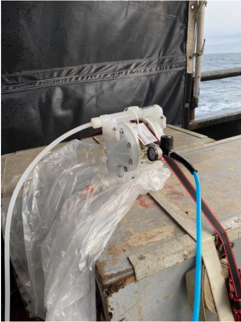
Close-up of pump with air regulator and air hose (blue) sitting on the mooring release pallets. It was necessary to use a ratchet strap to stabilize the pump so it did not move during sampling. Plastic bags were used as an extra precaution against contamination.
