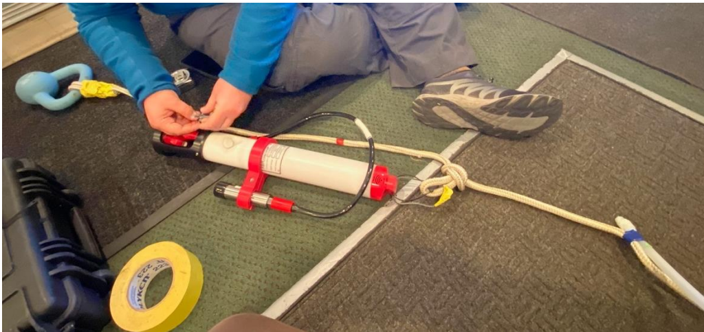
Trace metal tubing (far right) attached <1m above RBR CTD (middle) and ~2m from weight (far left).
