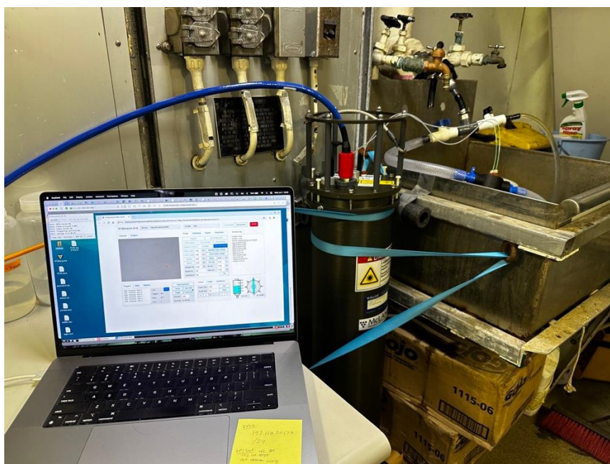
Picture of the IFCB set-up on Norseman II in 2022 (the IFCB is just the large black cylinder on the left of the picture). None of the other equipment pictured here is required for the IFCB to function, other than the white bucket for the water to be gathered:
